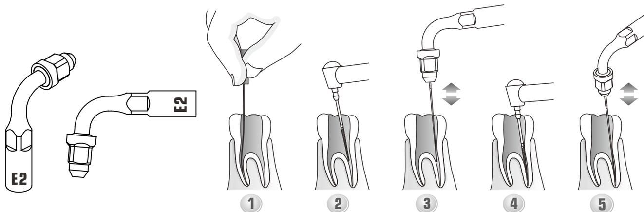
Use only the provided flat wrench to tighten the file holders on the handpiece, as well as for gently tightening the files or instruments in the holder. Do not over tighten.
